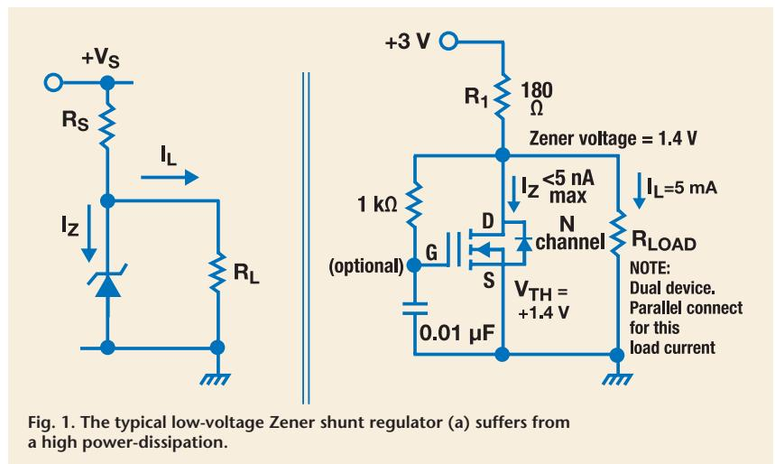
Fig. 1. The typical low-voltage Zener shunt regulator (a) suffers from a high power-dissipation.
