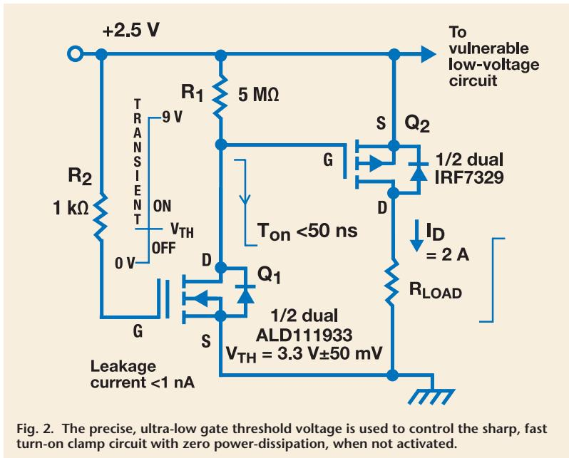
Fig. 2. The precise, ultra-low gate threshold voltage is used to control the sharp, fast turn-on clamp circuit with zero power-dissipation, when not activated.
